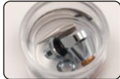
**4c.** Using an extra small cleaning brush dipped in Medea Airbrush Cleaner, scrub your nozzle, nozzle head cap, needle cap and nozzle cap.
