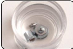
**4c.** Using an extra small cleaning brush dipped in Medea Airbrush Cleaner, scrub your nozzle, needle cap and nozzle cap.
