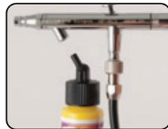
**1b.** Fill a clean bottle (not included) with Medea Airbrush Cleaner or water (depending on your media) and attach it to the airbrush.
