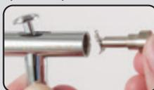
3. Reassemble by putting the trigger in first. **Make sure the opening on the trigger stem is facing front to back in the airbrush body.** Then screw on the needle chucking mechanism - auxiliary lever up.
