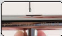
2. Put a tiny drop of Super Lube on the blunt end of the needle. Insert blunt end through the trigger opening and into the piston packing hole. Move needle up and down and in a circular motion to lubricate the o-ring.
