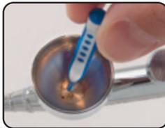
**3c.** Dip an Iwata Pipe Cleaner into a small cup of Medea Airbrush Cleaner.
